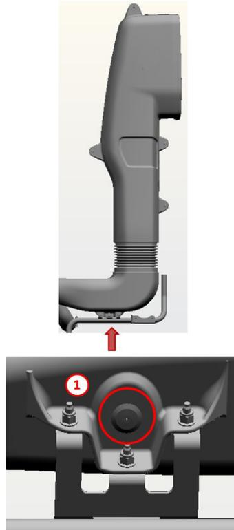
Press on the air filter valve (1) and filter inlet pipe valve (3) from their external surfaces and ensure that the dust and mud inside the valves is drained. Normal position of the valves is the closed position. Do not leave the valves at continuously open position.
