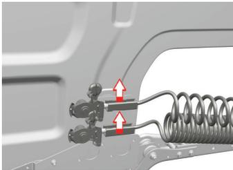
Remove the coupling hoses from their hangers before tilting the cab and do not tilt the cab while the coupling hoses are hanging.
