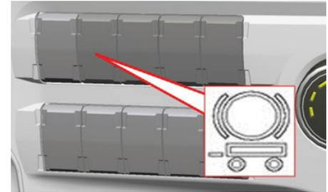
This brakes the semi-trailer only while attaching or detaching the semi-trailer, thus facilitates the attaching and detaching operations. If the
