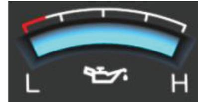
Indicates engine oil pressure in "bars". Oil pressure varies according to the oil temperature and engine speed
