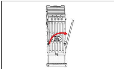
Open the upper connection profile of the step bracket under the battery cover in the direction of the arrow.
