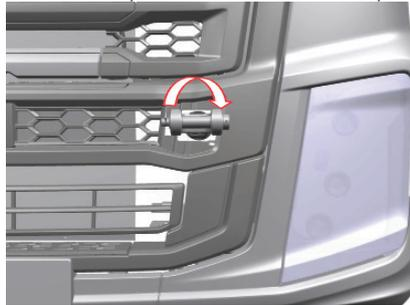
Install draw pin by rotating it clockwise as shown in the figure.
