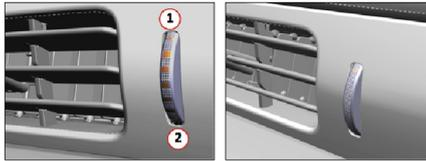
Use the control wheel to take adequate amount of air to the cab. Blowers on the driver and passenger sides have two positions, namely off and on. Air flow may be set as desired between these positions and the air flow may be directed vertically or horizontally using the setting feature on the center of the blower. Bring it to position 2 for maximum air flow.
