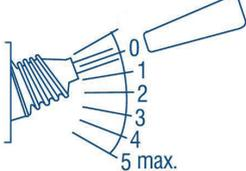
Intarder is activated by the 5 step lever on the right of the steering.
