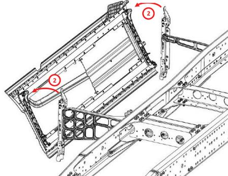
Side skirt panel is moved to the outwards of the vehicle on direction 2 after it is released of its locks.
