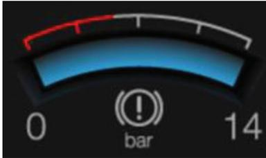
There are 2 independent air system circuits that supply for the front and rear brake systems. You can read the pressures of these systems from a single air pressure indicator.
