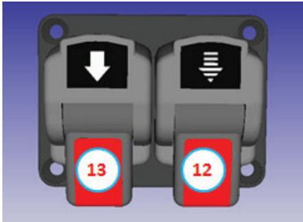
Control unit is used for lowering the bed in dump trucks. Button #12 is used for slow lowering, button #13 is used for fast lowering operation. Use the 'PTO (power take-off)' button in the panel to raise the bed.
