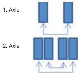
Wheel surfaces of your vehicle are polished specially and coated with protective transparent paint. Use your wheels in their original positions only. Or observe the following replacement chart. A wheel replacement other than the application specified below shall cause appearance problems.
