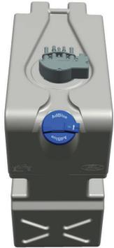
Your Ford Trucks vehicle with Euro6 emission system is equipped with an Urea system.
