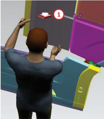
Side shroud is opened by holding it from the top and bottom as shown in the figure and then pulling it to the outside (2) of the vehicle and then to the front (2) of the vehicle.
