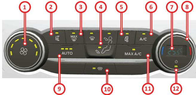
**1- Blower speed control:** Adjusts the amount of air to be blown to the interior of the vehicle.
