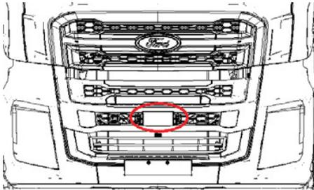
A message is displayed when the radar signals taken from the sensor are blocked by an object. The sensor is located behind the grille. When the sensor is blocked, the system cannot detect the vehicle in front, and thus cannot operate.
