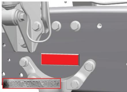
Chassis number is located under the front bonnet and on the chassis right hand-hand side arm and on the right chassis lower flange beside the engine crossmember; it consists of 17 digits. Example: NMOK13TEDFBL12345
