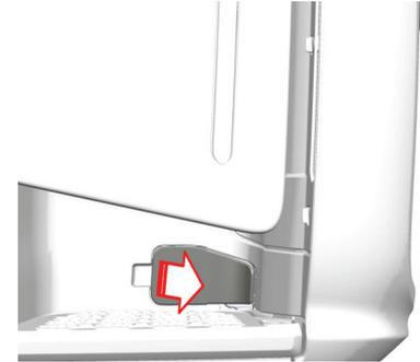
Cab tilt cylinder is located under the cover behind the step on the right side of the vehicle.
