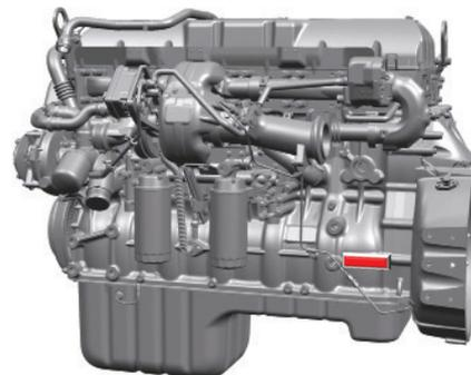
Metal label with the engine type and serial number inscribed on it is placed on the lower right side of the turbocharger intake pipe.
