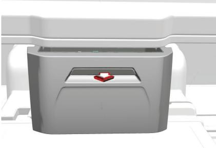
There is a one compartment drawer in the bed area. Pull it towards you to open it. The capacity of the under-bed storage compartment is 45 kg without a refrigerator and 30 kg with a refrigerator.
