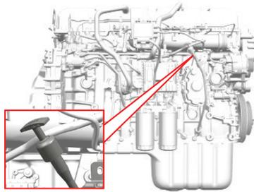
Engine oil level shall be inspected weekly. Engine oil dipstick is placed on the right side of the vehicle.
