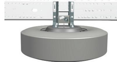
Spare wheel is on the left side of the chassis on vehicles with single fuel tank. To remove the spare wheel from its seat, loosen four bolts connecting it to the holder with the 24 spanner on the toolbox. Spare wheel is hanged with a cable. To release the cable, install the wheel brace to the rotating arm. Turn the brace anticlockwise.
