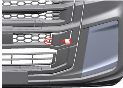
Press the draw pin cover from the side shown with an arrow. Cover shall rotate and open. Place it on its seat on the vehicle and press on it to install the part.
