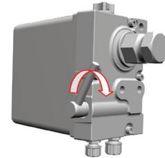
b) Lower the latch on the cab tilt cylinder down
