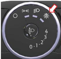
When the lighting control is on automatic headlamp position, low beam headlamps are turned on automatically when it gets dark on the evening and sensor detects that the ambient lighting level is not adequate.
