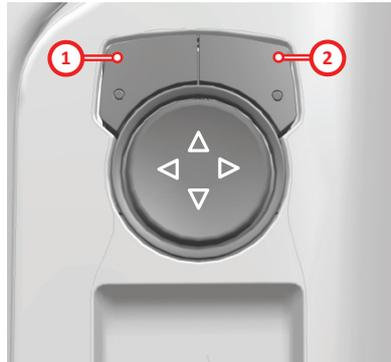
Press button no. 1 for the adjustment of the driver's side mirror. Adjust the mirror by moving the arrows forward and backward and left and right, then press button no. 1.
