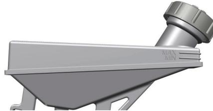
Clutch fluid reservoir is placed under the front hood. The level of fluid shall be up to the level mark on the reservoir.
