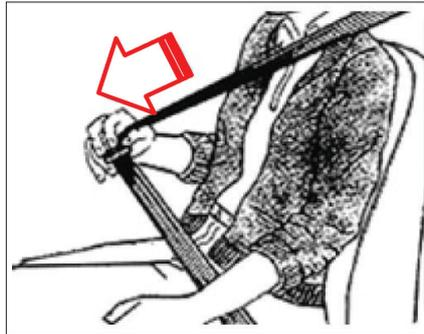
Pull the seat belt continuously from the reel. Seat belt may be locked when it is pulled too fast or when the vehicle is on a slope. In this case, relieve the seat belt and allow it to retract a little, then try again. Hear the locking click when you are inserting the latch of the seat belt to the buckle. Otherwise, seat belt is not locked. Adjust the height of the seat belt as per your your shoulder. (If height adjustment feature is available)
