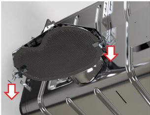
Put on a pair of gloves before installing spark arrester as the muffler is hot. Hook the spark arrester from its clips to the hangers in the muffler. Close the clips and retain the spark arrester to the exhaust.
