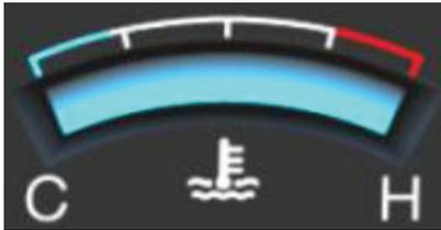
Indicates engine coolant temperature. If the dial of the indicator is in the red area, the engine may overheat.
