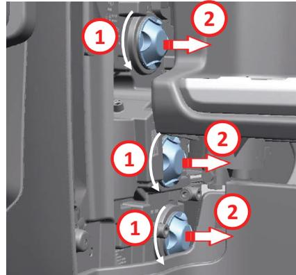
Remove the cover by rotating it counter-clockwise and unlocking it for the main beam on the top, dipped beam in the center and fog lamp at the bottom.
