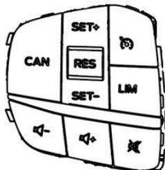
Speed controls are located on the steering wheel.
