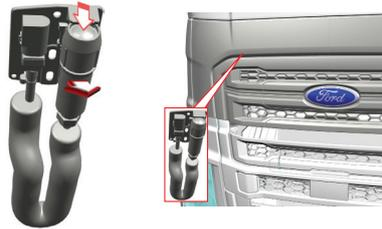
2) Press and hold the cab tilt button under the bonnet. The cable of the button is flexible. Tilt the cab by moving to the side of the vehicle.
