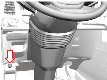
1. Press the button on the lower left side of the steering column with your foot. Thus, power assist to the system shall be activated and setting shall be allowed.
