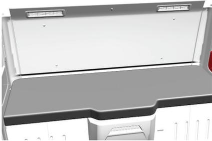
There is a foldable compartment at the right end of the lower bed. Pull the handle up to raise the compartment. Pull the handle up to the top and release it to lower the compartment.
