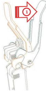
Side skirt panel is released of its locks with the movement of the locks on both front and rear sides to the direction of 1.
