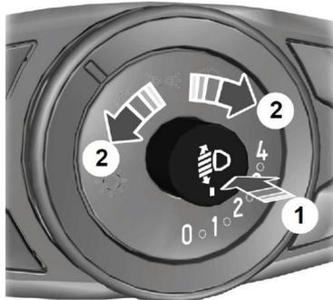
Press the button on the headlamp switch to make it come out.
