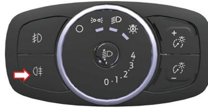
Rear fog lamp switch is placed on the headlamp control panel. Turn this switch on to obtain better visibility and be visible to the incoming traffic in foggy conditions and where the visibility is low. Rear fog lamps are illuminated when the low and high beam headlamps are activated only. Rear fog lamp icon is displayed on the indicator when the switch is pressed.
