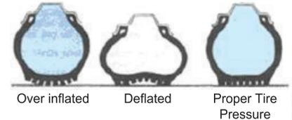
Low pressure cause wear on the shoulder areas of the tire. High pressure cause wear on the back areas of the tire.
