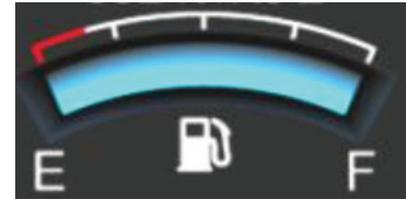
Indicates the fuel level in the tank Yellow warning light indicates that the fuel in the tank is reduced. Refill fuel immediately. System will take air if the fuel is lowered.
