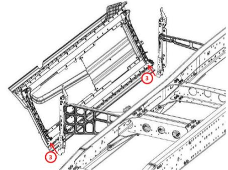
Side skirt panel is moved to the upwards on direction 3 after it is released from the rope hooks on the front and rear sides and it is released from its hinge connections.
