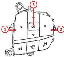
Trip computer shows the information and the warnings. Trip computer data may be changed by the control panel on the steering wheel.
