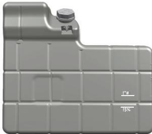
Engine coolant contains 50% antifreeze and 50% distilled water. Coolant circulates inside the engine block and cools the engine components. This fluid also cools the intertarder oil in vehicles with intertarder.
