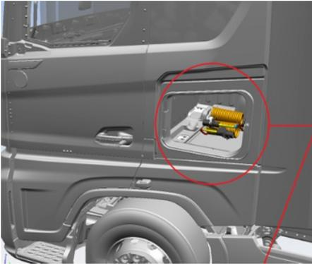
Trailer installation kits located in the trunk of your vehicle should be kept in the trunk or inserted into the parking sockets when not in use.
