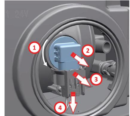
Remove the bulb by rotating it counter-clockwise and unlocking it to replace the fog lamp bulb. Then, release the bulb by pulling the connector tab out. Place the new bulb to its seat after installing it to the connector and lock by rotating clockwise.
