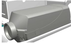
Eberspacher airtronic D2 dry type heater is used. This device is placed under the lower bed inside the cab. On/off switch is located on the front console and the right wall of the lower bed. Detailed settings may be performed on the instrument panel. Auxiliary heater can also be operated when the ignition is off.
