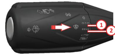
Wiper lever “Automatic wiper” position If your vehicle is equipped with an Automatic Wiper, wipers shall operate automatically as per the amount of rain when you bring the wiper lever to “Automatic Wiper”
