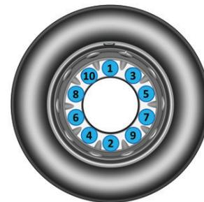
Check the wheel nut torque when you load the vehicle with full load for the first time. (750 Nm +/- 50Nm for front and rear wheels) Tighten the wheel nuts alternately.
