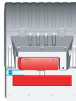
In tractor vehicles, the distance between lower side of the stop lamp on the rear left fender and upper side of the license plate's sheet plate.
