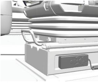
Chassis height of the vehicles with air bellows on rear axle may be adjusted by the control.
