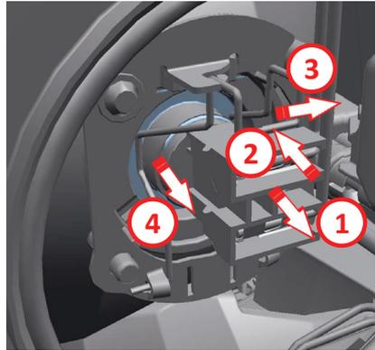
Remove the connector behind the bulb by pulling it out first to replace the dipped beam bulb. Then, press on the retaining spring wire and release and open it from the by sliding to the right-hand side and remove the bulb. Insert the spring to the tab and install the bulb connector after placing the new bulb.
