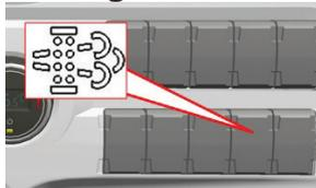
The button on the center console shown above is intended for manual exhaust cleaning. You can perform manual exhaust filter cleaning of the vehicle using this button.
