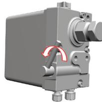
b) Lift the latch on the cab tilt cylinder up.
