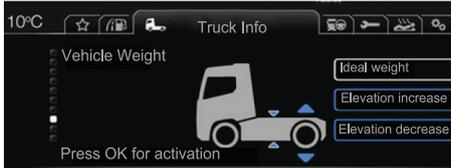
5. Check the warning colour when "ECAS warning active" message is displayed on the Display Screen. Error is critical and no ECAS function shall operate if the red warning is active. ECAS functions resume to operate manually or as limited as per the status of the error if the yellow warning is active. However, we recommend you to drive to the authorized service in both cases.
