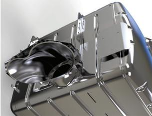
Spark arrester shall be installed at hazardous material loading, unloading locations and fuel stations during fuel filling or draining. When the vehicle is out of the station, the spark arrester shall be removed.
