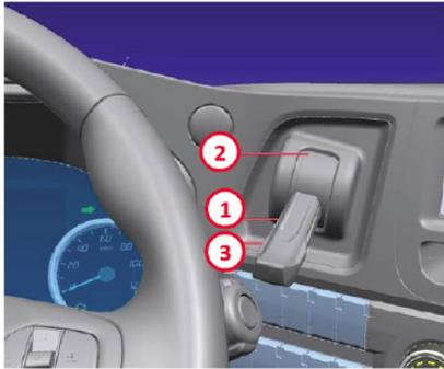
Bring the park brake lever to position 1. When the park brake is engaged, the display flashes red.
