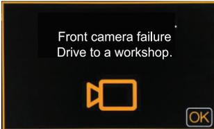
**Note:** If you see the following warning on the instrument panel, you shall take your vehicle to a Ford Authorized service. The Lane Departure Warning System shall not be active until the vehicle is inspected by the service.
