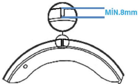
Lining wear inspection may also be performed visually from the inspection holes on the brake dust plate.
