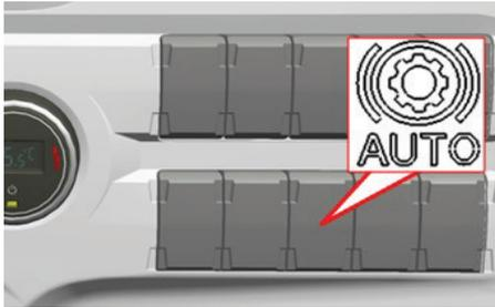
When the “AUTO” button on the center console is pressed, intarder and engine brake may be activated by the foot brake. Thus, when the brake pedal is applied, intarder\* and engine brake is applied as proportional to the pedal travel besides the service brakes. \*intarder is not provided in standard vehicle package; it is optional.
