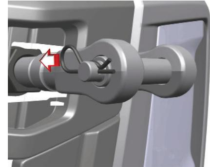
Remove the draw pin and attach the towing cable.
