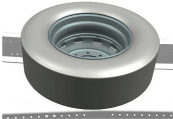
Spare wheel is on the chassis on vehicles with an optional secondary fuel tank. Side skirt shall be removed to take the spare wheel out.
