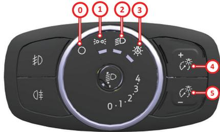
Headlamp switch is placed on the console to the left of the steering.
