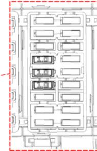
The diodes shall be fitted into the slots in clockwise order with a value of 1.0 shown on them.
