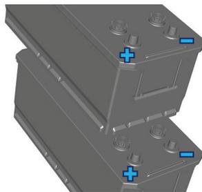
Disconnect the terminals after 5 minutes minimum when you stop the engine. This is needed to supply power to the Urea system that will operate after a while when the engine is stopped. Otherwise, your Urea system (or vehicle) may be damaged.
