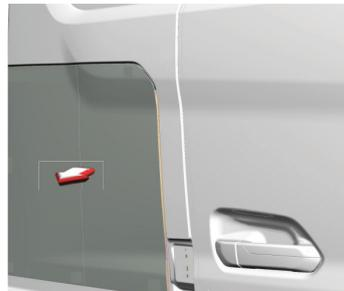
Toolbox is located behind the driver and passenger doors as shown in the figure.
