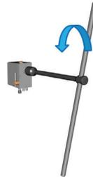
c) Rotate the hexagonal bolt on the cab tilt cylinder in the direction of arrow until the cab is tilted completely with the wheel nut spanner delivered in the toolbox of your vehicle.
