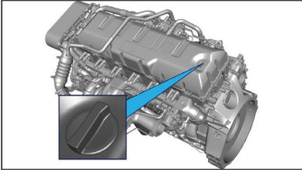
Add oil if the level is less than MIN, engine oil filler cap is on the cylinder head cover. Wipe the surroundings of the cap before opening it. Pay attention to cleanliness if you would use equipment such as measuring container, funnel etc.
