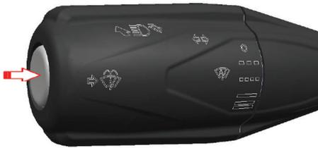
Press the button shown with an arrow on the left multifunction lever to spray wiper fluid to the windshield. Spraying function shall be stopped when you release the button.
