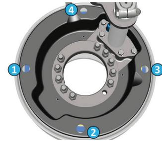
Z-cam brake system is a lining-drum type braking system. Brake lining wear is inspected from 4 holes on the brake plate. Remove the plugs on the plate for inspection, and replace them after inspection.
