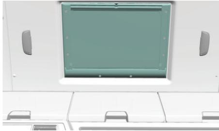
Power roof moves to opening or closing direction while the opening/closing buttons are pressed. Operation is stopped automatically when the power roof reaches uppermost or lowermost position. Buttons are active while the ignition is on. Power roof is closed automatically when the control switch is pressed once for a short period while it is open. Power roof is opened automatically when the control switch is pressed once for a short period while it is closed.
