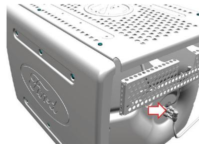
Various sensors and urea injector shall be available on the exhaust muffler. When you wash your vehicle, do not apply water jet on the urea injector on the muffler, sensors and the electric connections. DOC, DPF and SCR catalyst are available in the exhaust muffler. These parts are ceramic-based bricks, and it is definitely not allowed to wash these parts. Do not attempt to wash inside the muffler from the muffler outlet or from the injector housing by removing the urea injector.
