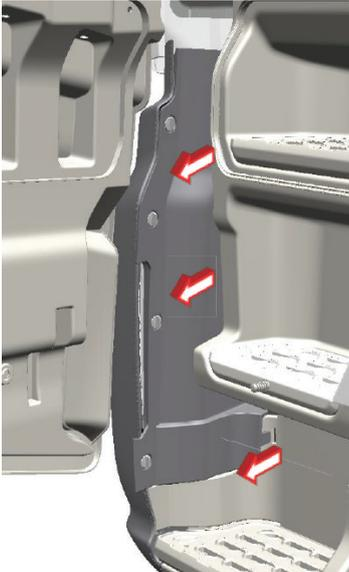
Release the part from its seat on the bottom and remove it.
