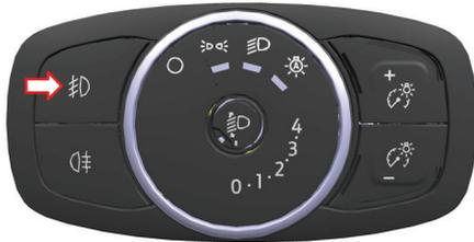
Front fog lamp is placed on the headlamp control panel.
