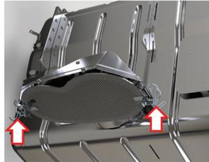
Put on a pair of gloves before removing spark arrester as the muffler and spark arrester is hot. The spark arrester is removed from the exhaust pipe by loosening the brackets on it.
