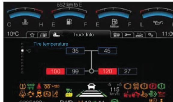
Stop the vehicle safely, inspect the tires and inflate them to correct pressure if the tire pressure low warning lamp is lit. This system does not replace correct tire maintenance procedures.
