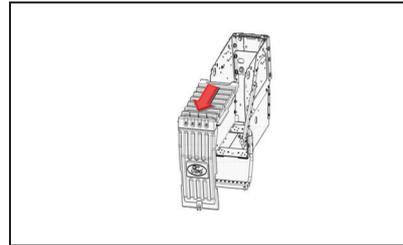
Then pull the battery cover to yourself in the arrow direction and remove easily.
