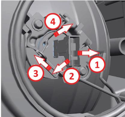
Remove the connector behind the bulb by pulling it out first to replace the main beam bulb. Then, press on the retaining spring wire and release and open it from tabs by sliding to the upper left side and remove the bulb. Insert the spring to the tabs and install the bulb connector after placing the new bulb.
