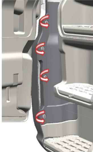
Open the door, rotate the removable locks on the part in the direction of the arrow.
