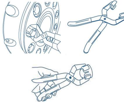
Remove the wheel nut caps with the special pliers provided in the toolbox of the vehicle for aluminum alloyed wheels.
