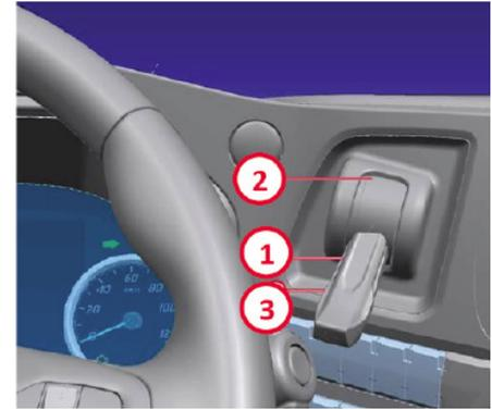
After taking lever to position 1, check whether the vehicle with semi-trailer moves by pressing on the lever and pulling the lever down (position 3). Then, bring the lever to park position (position 1) again. Then, get off the vehicle and apply the trailer park brake.
