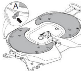
The surface of the platform should be greased with a sufficient quantity of durable, high pressure <NLGI Class 2> grease containing MoS2 or graphite additives prior to the first attachment of a trailer.
