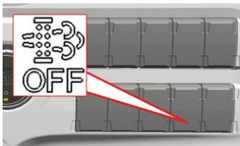
The button on the center console shown below is the exhaust filter cleaning prevention button. You can prevent the exhaust filter cleaning of the vehicle using this button. When exhaust filter cleaning is prevented, the instrument panel shall display "Exhaust filter cleaning is prevented by the driver" warning. The detailed explanation about this warning can be found in the warnings section.
