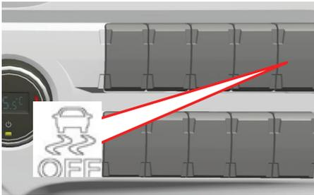
You may want to disable ESP on soft road conditions. In this case, press the ESP cancel switch located in the centre console.
