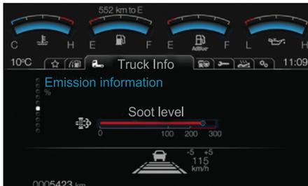
If the exhaust level is above 100%, the part between 0% and 200% of the bar will blink.
