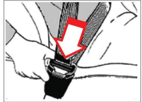
**Press the red button on the buckle to release the seat belt. Then, release the belt slowly to allow that it is wound on the reel fully.**
