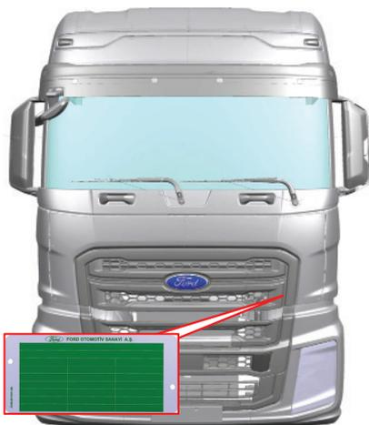
Vehicle identification plate is located under the hood in the front of the cab.
