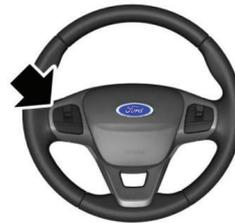
Controls of the adaptive speed control system are located on the steering wheel.
